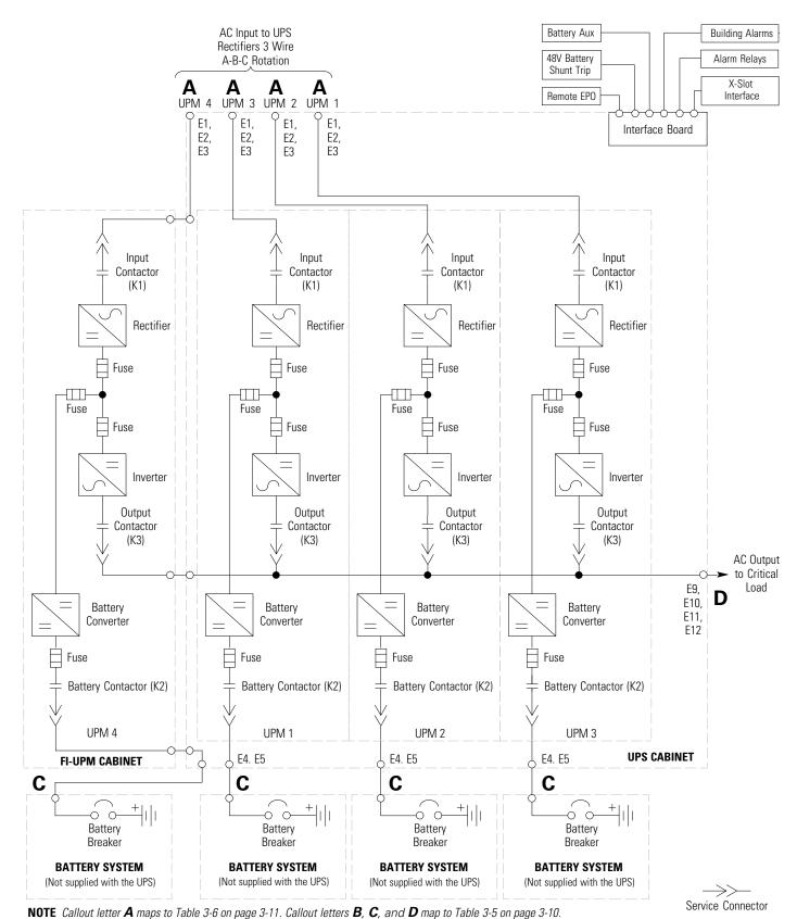
Figure 6-16. Plus 1 UPS System – Separate Rectifier Feed, Separate Battery, IOM Configuration
